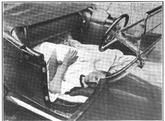
View showing the method of converting roadster into sleeping car
